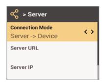
• Connection Mode: When you select Device -> Server, you can send a connection signal from the device to a server with the input information directly. When you select Server -> Device, Server IP and Server Port cannot be entered.
